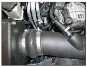
16. Connect the factory crank case vent hose to the quick disconnect fitting installed into the AIRAID<sup>®</sup> intake tube.
