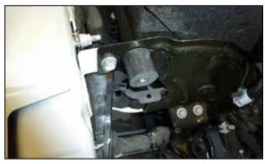
12. Install the provided rubber mounted stud into the fender bracket as shown.
