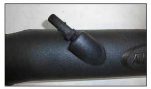
7. Install the provided quick disconnect vent into the AIRAID<sup>®</sup> intake tube as shown.
