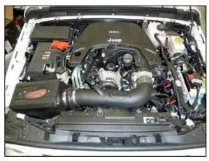
17. Double check your work!Make sure there is no foreign material in the intake path.Make sure all clamps, hoses, bolts, and screws are tight.Double check the hood clearance!Reconnect the negative battery cable!
