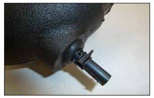
6. Install the provided grommet into the AIRAID® intake tube. Remove the inlet air temperature sensor from the factory intake tube, Remove the O-ring from the sensor and then install the sensor into the grommet installed into the AIRAID® intake tube. NOTE: Use caution while handling the inlet air
