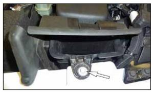
4. Remove the bolt that secures the fresh air duct to the inner fender and remove the factory air box. NOTE: AIRAID recommends that customers do not discard factory air intake.
