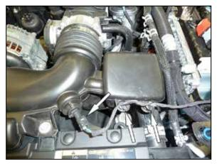
2. Disconnect the inlet air temperature sensor electrical connection and unhook the wiring harness from the intake plenum.
