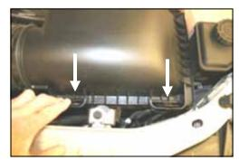
**3.** Pull both lockdown tabs towards you on the factory airbox lid to remove the lid from the base.
