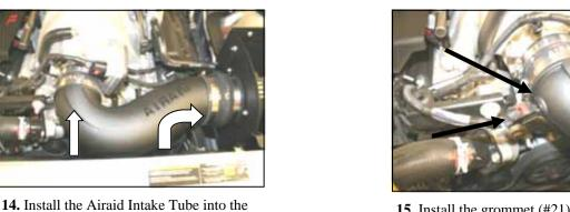
**15.** Install the grommet (#21) into the hole in the Airaid Intake Tube, and then gently push the temperature sensor (*removed in step #4*) thru the grommet until completely seated.
