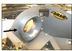
**8.** Next install the filter adapter (#6) using three 1/4 - 20 button head bolts (#12), and 1/4" flat washers (#13).
