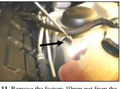
**11.** Remove the factory 10mm nut from the stud on the driver's side inner fender and save it for the next step.
