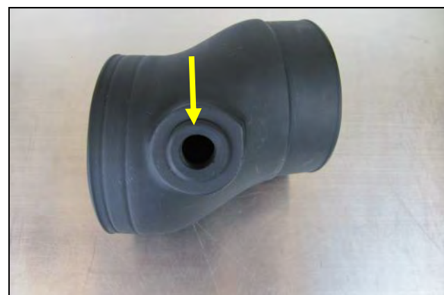
6. Insert the Grommet into the Intake tube. NOTE: On some models the CCV hose does not connect to the factory air filter housing but connects to the intake tube near the throttle body. On these models install the provided plug into the intake tube in place of the grommet.
