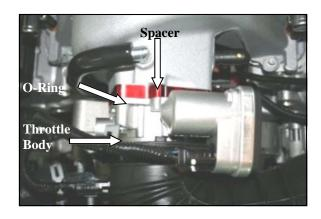
3. Install the O-Ring (#2) into the groove on the Poweraid Spacer (#1). Install the spacer between the intake manifold, and the throttle body with the O-Ring facing the throttle body. Insert four 6mm x 60mm Hex Bolts (#3), and 6mm Flat Washers (#4) through the throttle body, Poweraid Spacer, and into the intake manifold. Using a 10mm socket, tighten all 4 throttle body bolts evenly, to the manufacturer's specifications.
