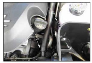
13. When equipped, secure the PCV Hose on both ends using the two Speed Clamps.
