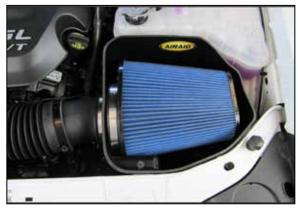
14. Install the Airaid Premium Filter onto the Filter Adapter.
