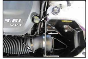
12. When equipped, slide the factory intake tube onto the Airaid Tube, adjust if necessary and tighten the Clamps. Connect the crank case breather line to the Barbed filling using the supplied PCV Hose.
