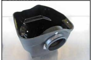
5. Slide the Coupler and Clamp onto the Filter Adapter as shown. Do not tighten the Clamp at this time.
