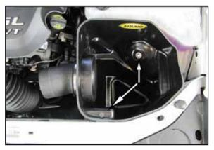
11. Lower the Air Box assembly down into the inner fender. Align the bolt holes and secure the Air Box using the screw removed in step 3 and the 3/8" Button Head Screw with the 5/16" Flat Washer.
