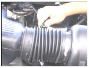
**3.** Remove the crankcase breather hose from the factory intake tube and the valve cover. Disconnect the Air Intake Temperature (AIT) sensor wiring harness from the sensor. (4.6L Engine only: Disconnect the Idle Air Bypass Valve (IABV) inlet tube from the factory intake tube.) (5.4L Engine only: disconnect the IABV, save the plastic hose for reuse.)
