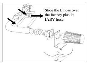
13. <u>5.4L engines</u>: Measure and cut the 3/4 x 12" L-hose (#7) as needed, then slide it over the factory plastic **IABV** hose. Install the hose onto the Airaid Intake Tube nipple and secure it using two #22 speed clamps (#17).
