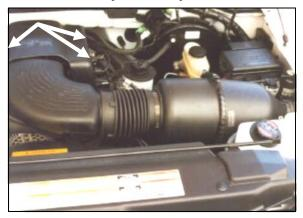
**1.** <u>Disconnect the negative battery cable.</u> Using a 10mm socket, remove the three bolts securing the engine beauty cover, remove the cover, and set it aside (save the bolts and cover for reuse).
