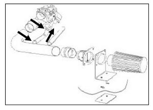
15. <u>4.6L engines continued</u>: Connect the Airaid Intake Tube nipple to the *IABV* inlet tube using the 3/4 x 1/2" L-hose (#7), and two #22 speed clamps (#17).
