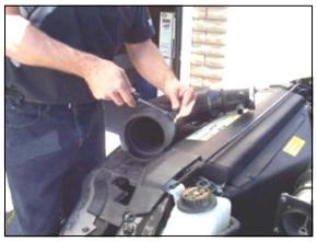
**4.**) Remove the factory intake tube, and set it aside. Remove the **AIT** sensor from the tube by carefully prying it out with a flat blade screwdriver (save the sensor for reuse). Disconnect the **M**ass **Air Flow**
