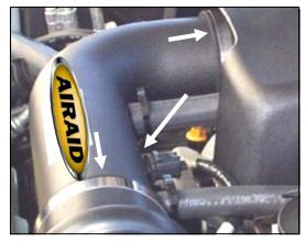
11. Install the 7/16" rubber grommet (#15) into the Airaid Intake Tube (#2). Insert the factory AIT sensor into the grommet. Slip the Airaid Intake Tube into the urethane hump and reducer hoses. Align for best fit and tighten the remaining hose clamps. Tighten the MAF bracket and reconnect the AIT sensor wiring harness. Apply the Airaid Bubble Decal onto the Intake Tube
