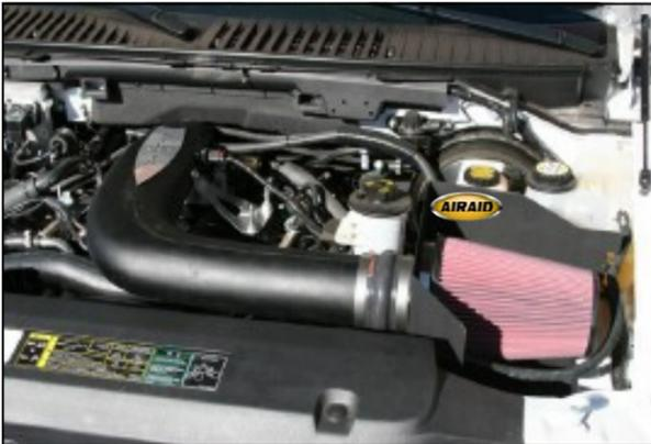
16. Install the Airaid Premium Filter inside the cold air dam. Apply the Airaid Foil Decal onto the Panel as shown.
