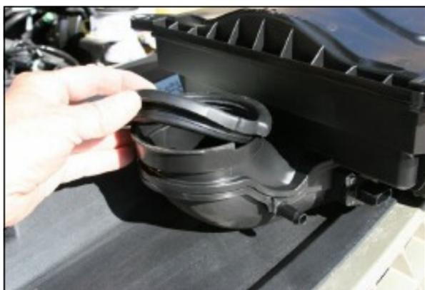
**7.** Remove the factory rubber seal from the airbox, and install it on the Airaid intake tube.
