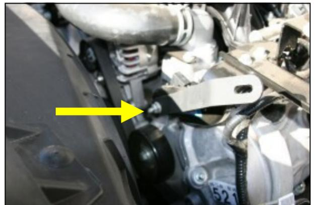
**3.** Remove 13mm nut on power steering reservoir bracket. Install Airaid intake tube support bracket, replace nut, and leave slightly loose. (Nut will be tightened after final adjustments.)
