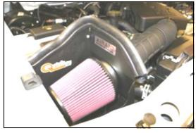
**13.** Install the Airaid Premium Filter (#1) into the **MAF** adapter, and tighten the hose clamp. Next install the weather strip (#5) onto the top of the Quick Fit Panels as shown.
