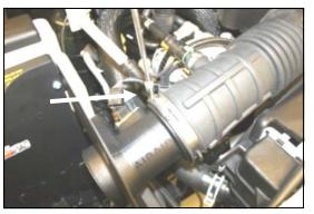
**11.** Reconnect the factory intake tube to the Airaid **MAF** adapter, and then tighten the hose clamp.
