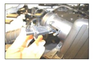
6. Using the supplied #20 Torx bit, remove two screws, and remove the Mass Air Flow sensor
