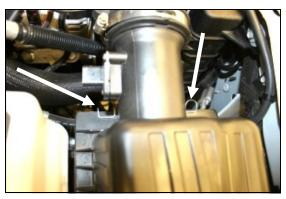
**3.** Unlatch the two metal clips that hold the factory air cleaner lid to the base.
