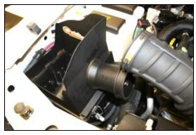
**10.** Install the Quick Fit Assembly onto the top of the factory air cleaner base. Start by sliding the three tabs on the Airaid panel thru the three slots on the top of the base. Center the panel assembly, and re-latch the two factory clips.
