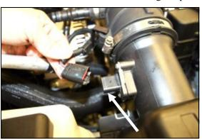
2. Slide the red tab on the bottom of the Mass Air Flow sensor wiring connector and then squeeze the connector, and unplug the harness from the sensor.
