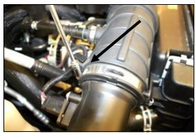
1. **Disconnect the negative battery cable.** Loosen the hose clamp that holds the factory intake tube to the air cleaner lid.
