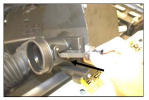
**9.** Reinstall the factory **MAF** sensor removed in step #6, into the Airaid **MAF** adapter as shown using two 8-32 button head screws provided in the kit. **Do Not Use The Factory Screws!!**
