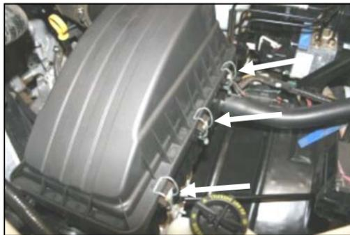
**2.** Unlatch the three metal clips that hold the airbox lid to the base.
