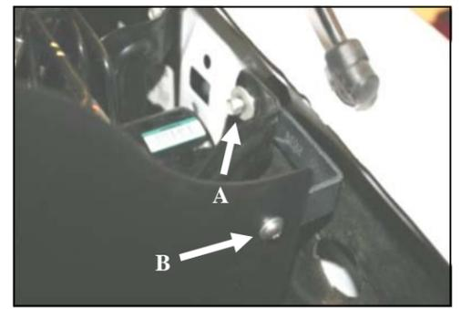
**12. A.)** Slide the L-bracket under the anti lock braking system bracket, and re-install the bolt removed in step #8. **B.)** Fasten the bracket onto the back of the panel using one 1/4-20x1/2" button head bolt (#6), washer (#7), and serrated nut (#8). Tighten securely.
