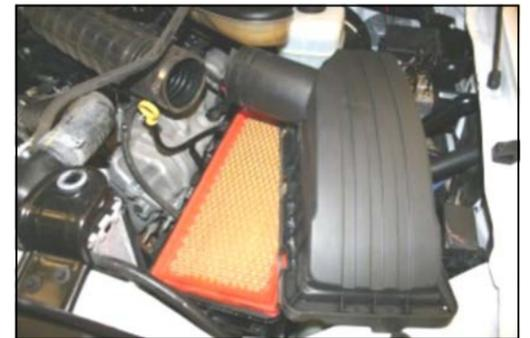
**3.** Remove the airbox lid and air filter from the vehicle.
