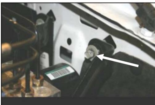
**8.** Using a 10mm socket, remove one bolt which secures the anti lock braking system bracket to the drivers side inner fender. The bolt will be reused in step #12.
