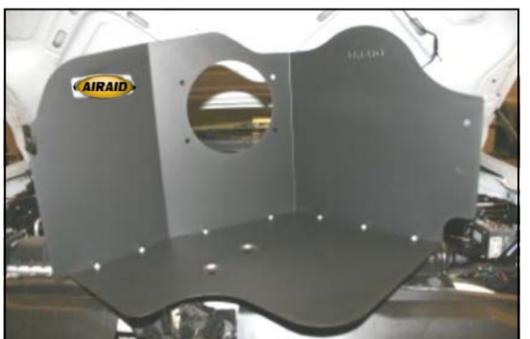
**9.** Assemble the two Cool Air Dam panels (#2 and #3) as shown, using seven 6-32 screws (#10), #6 washers (#11), and keps nuts (#12). Tighten securely. Apply the Airaid Foil Decal onto the Panel as shown.
