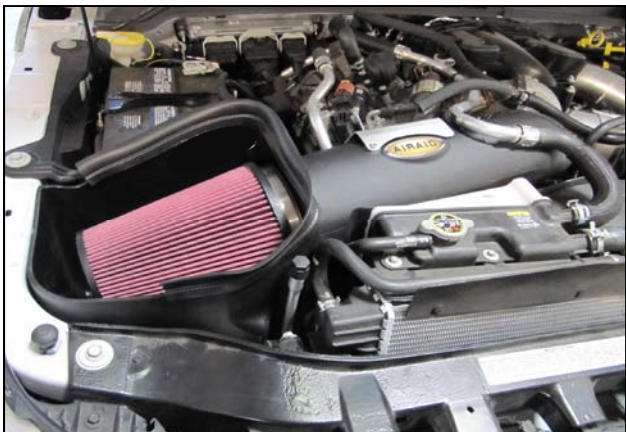
18. Install the Airaid Premium Filter inside the CAB and complete the install by trimming the CAB with the Weather Strip.
