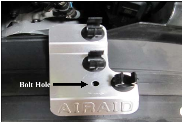
15. Insert the three remaining Hose Anchors into the Hose Bracket as shown.
