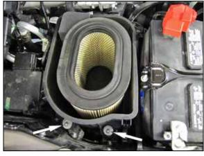
4. Remove the two bolts that secure the lower air filter housing to the mounting bracket, then pull the lower air filter housing straight up to dislodge it from the mounting grommets and remove it from the vehicle.
