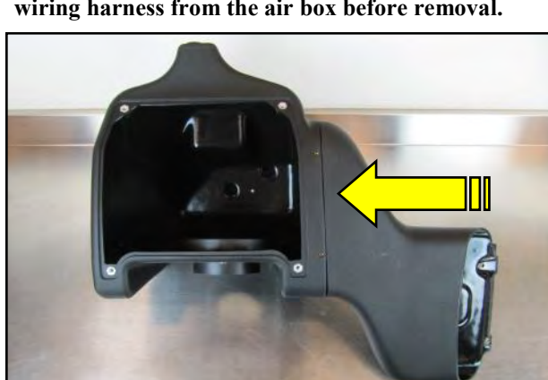
8. Snap the new Air Scoop into the Airaid Air Box as shown.
