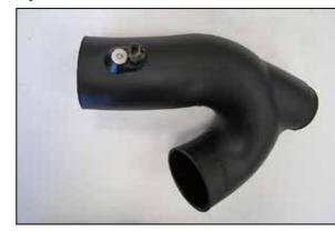
19. Install the inlet air temperature sensor into the AIRAID® intake tube and then secure with the provided hardware.
