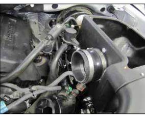
16. Install the coupler hose onto the filter adapter and secure with the provided hose clamp.
