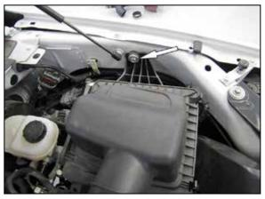
5. Remove the bolt which secures the factory air filter housing to the inner fender. Remove the factory air filter housing and fresh air intake from the vehicle.
