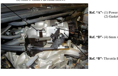
Ref. "C"- (2) 1" Linkage Plates (2) 6mm x 12mm Flat Head Screws
