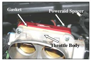
3. Install the supplied gasket between the throttle body, and the Poweraid Spacer. Use caution to retain the factory o-ring in the groove on the intake manifold. Slide two of the supplied 6mm bolts and washers thru the top holes of the throttle body and into the manifold.
