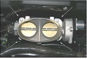
2. Using a 8mm socket, remove four bolts that hold the throttle body to the intake manifold.
