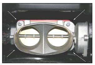
4. Next install the remaining two bolts and washers thru the throttle body and into the manifold. Tighten all four bolts evenly to the manufacture's torque specifications.
