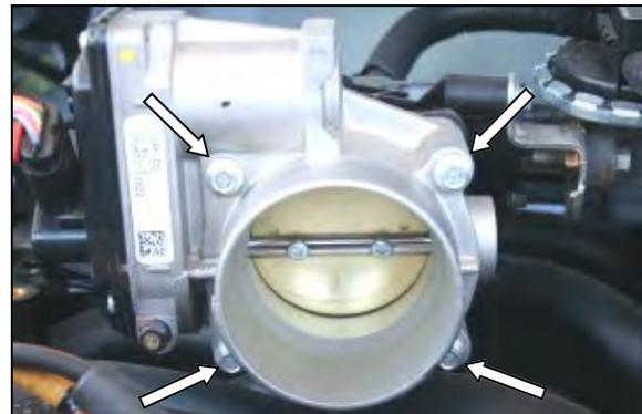
2. Remove the four bolts (and/or nut and stud) from the throttle body, and remove the throttle body from the intake manifold, and set it aside. Retain the wiring harness anchor from the upper left stud on the Explorer for reinstallation in step #4.
