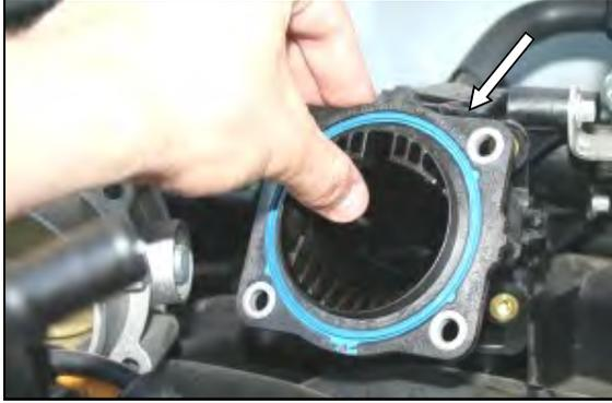
3. Remove the factory black plastic spacer that is located between the throttle body and the intake manifold.
