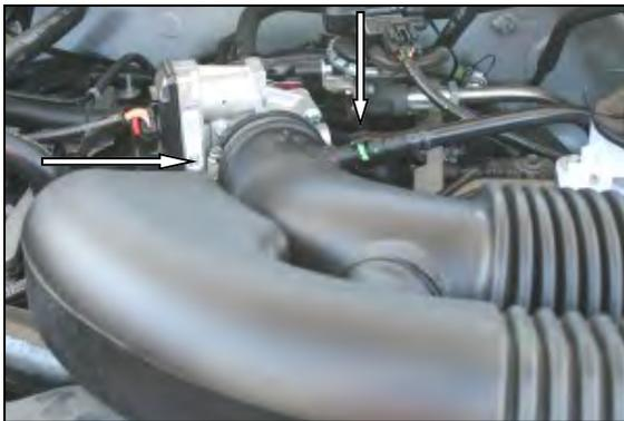
5. Re-install the factory intake tube onto the throttle body and tighten the hose clamp. Re-connect the breather hose to the factory intake tube.
