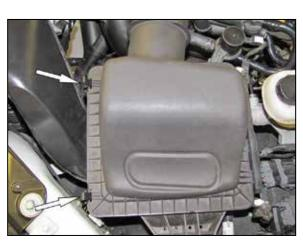
4. Release the two clips that secure the upper air filter housing and then remove the housing and factory air
