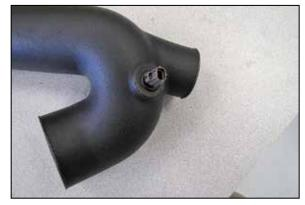
8. Remove the inlet air temperature sensor from the factory intake tube. Remove the O-Ring from the inlet air temperature sensor and then install the sensor into the AIRAID<sup>®</sup> intake tube using the provided grommet. **NOTE: Use caution while handling the inlet** temperature sensor as it is very fragile.
