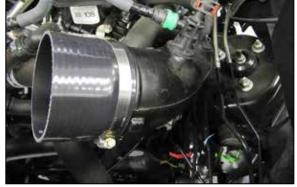
6. Install the provided coupler hose onto the turbo inlet tubes and secure with the provided hose clamps.
