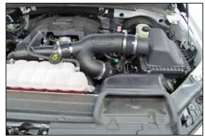
12. Double check your work! Make sure there is no foreign material in the intake path. Make sure all clamps, hoses, bolts, and screws are tight. Double check the hood clearance! Reconnect the negative battery cable!
