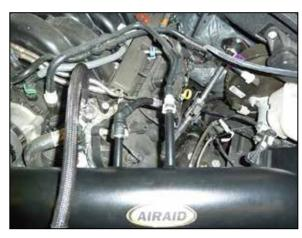
15. Connect the factory EVAP and Crank case vent lines to the fittings on the AIRAID $^{\otimes}$  intake tube.
