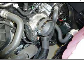
13. Install the provided coupling hose onto the throttle body and secure with the provided hose clamp.
