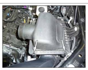
5. Release the two clips securing the upper air filter housing and then remove the upper filter housing and stock air filter.
