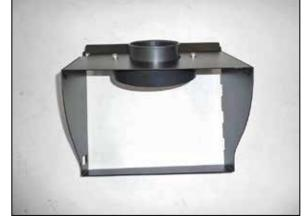
6. Install the filter adapter into the AIRAID $^{\otimes}$  heat shield and secure with provided hardware.
