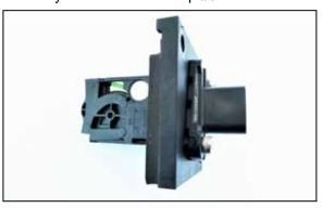
9. Install the gasket onto mass air sensor adapter and then remove the mass air sensor from the factory filter housing and install it into the adapter using the provided hardware.
