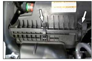
4. Release the three clips that secure the air filter housing lid and then remove the lid, intake tube and air filter from the vehicle.
