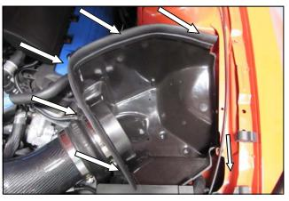
**14.** Install the Weather Strip (#8) onto the Cool Air Box with the contoured edge rolling away from the filter area. Start at the front of the vehicle and work your way back
