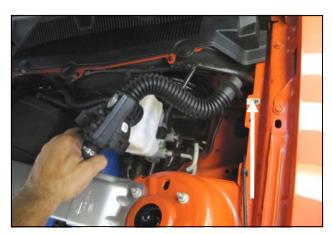
**4.** Unbolt the Intake resonator from the inner fender and disconnect it at the drivers side firewall. Remove the entire assembly from the vehicle and set it aside. It will not be reused.
