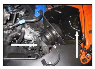
12. Install the **CAB** into the vehicle. Make sure that the air inlet of the **CAB** aligns with the factory duct, and the two locating pins on the bottom are seated in the factory grommets. Next reinstall the factory bolt that was removed in step #3 thru the steel sleeve and grommet and into the inner fender.
