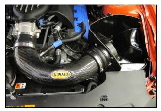
**13.** Install the Airaid Intake tube onto the throttlebody first then into the Hump Hose and tighten the clamps. Reconnect the crank case breather line to the Aluminum fitting on the Intake Tube.
