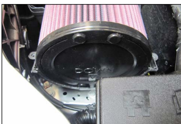
7. Install The Airaid Premium Filter and clamp into the air box as shown, with the Arrow pointing Down and the Lugs in the correct position. When properly installed, the Filter top will be completely inside of the airbox lower half.
