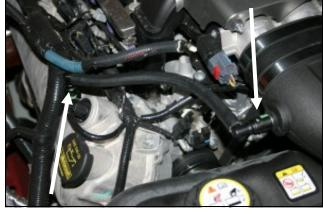
**16.** Install the two factory connectors from step #15 into each end of the supplied 3/8"x12" breather hose (#10). Now reattach one connector to the valve cover, and the other end to the aluminum fitting on the intake tube.
