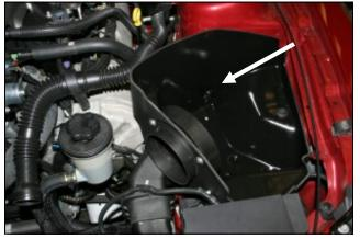
4. A.) Install the filter adapter (#9) using three 1/4-20 5. Turn the CAD so that the bottom faces the left fender 6. Install the CAD into the vehicle making sure that the and towards the front. The last anchor nearest the MAF was removed in step #2 thru the steel sleeve and grommet and into the inner fender. Make sure that the wiring harness is not pinched under the CAD.
