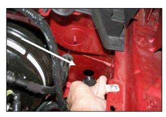
7. Install the optional firewall plug (#20 on the main page) into the hole in the firewall.
