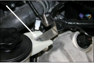
11. Install the bracket assembly from step #10 as shown. 12.A.) Install the oval coupler onto the intake tube This bracket and 6mm bolt will secure the power steering using two #72 hose clamps (#17). Leave the clamps loose reservoir and replaces the stud removed in step #9.
