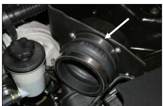
7. Install the provided hump hose (#5) onto the filter 8. Slide the Modular Venturi Tube (#3) into the Airaid 9. Lift up on the intake resonator tube to disengage it adapter using two #72 hose clamps (#17) as shown. intake tube (#2) making sure to align the two slots for Leave the two hose clamps loose for now.
