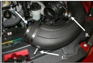
for now. **B.**) Install the 1 3/4" coupler (#7) onto the intake tube using two #28 hose clamps (#18) as shown. Tighten only the clamp against the tube for now. C.) Install the provided grommet (#19) into the intake tube and then install the aluminum fitting (#21) into the grommet as shown.
