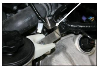
**3.** Using a 10mm socket, remove the resonator bracket from the power steering reservoir.
