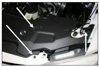
**10.** Reposition the plastic cover and then reinstall the three plastic trim anchors removed in step #6 into their respective holes and push down the center to secure the plastic trim panel.
