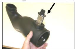
**12.** Align the two slots in the tubes, and install the factory mass air sensor removed from step #5. Make sure the screw holes line up, then install the two supplied button head screws. (#11).
