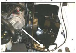
**8.** Place the **CAD** into the inner fender, align the bolt holes and re-install the bolt from step #6.
