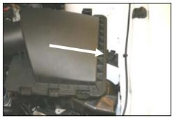
**3.** With a 10mm socket, remove the bolt holding the factory airbox to the fender and save the bolt. It will be reused
