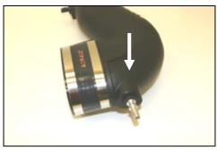
**13.** Install the oval coupler (#3) with two #72 hose clamps (#12). Tighten <u>only</u> the clamp closest to the aluminum fitting. (*Hint: For a clean look, locate the hose clamp tightening screws under the tube*)!
