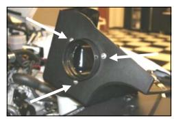
7. Install the air filter adapter (#5) into the Cool Air Dam (#7) as shown, using 3 button head bolts (#9) and 1/4" flat washers (#10).
