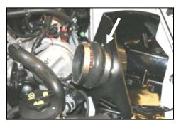
**10.** Install the hump hose (#4) on the filter adapter (#6), with two #72 hose clamps (#12). Tighten only the clamp next to the **CAD**.
