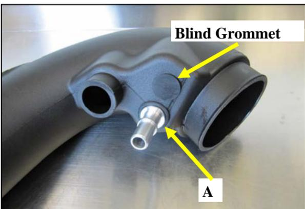
4. Install the Grommets and Fittings into the Airaid intake tube A) All models will require the use of the 5/8" Fitting (#19) and the 5/8" Grommet (#20). B) Automatic transmission equipped vehicles will also use the 3/8" Fitting (#18) and 3/8" Grommet (#21). Manual transmission vehicles will not need the 3/8" components and will use the Blind Grommet (#22).
