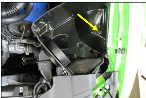
8. Install the Cool Air Box into the vehicle. Make sure that the Air inlet mates with the factory duct, and the two locating pins on the bottom align with the factory grommets. Next reinstall the factory bolt that was removed in step #3 through the steel sleeve and grommet and into the inner fender.
