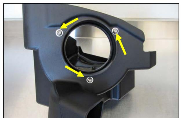
6. Install the filter adapter (#8) using three 1/4-20 button head bolts (#10), and flat washers (#11) into the Airaid Cool Air Box as shown.
