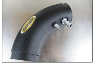
**5.** Install the Grommets and Aluminum Fittings into the Airaid Intake Tube. Apply the Airaid Bubble Decal onto the Intake Tube as shown.
