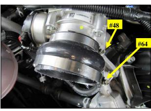
**14.** Slide the Reducer with one #64 and one #48 clamp onto the throttle body as shown.
