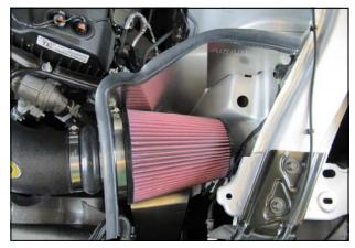
**18.** Install the weatherstrip on top of the Panel assembly as shown with the contour rolling away from the filter.
