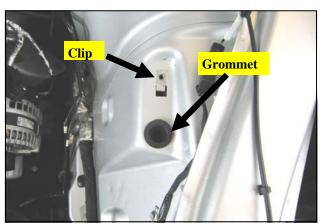
**4.** Be sure to retain the speed clip in the inner fender, but remove the grommet if it does not come out with the air box .
