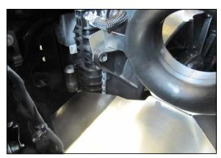
12 When properly installed, the Panel tab resides behind the fan shroud as shown.
