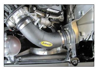
**15.** Install the Airaid Tube into the Hump Hose and Reducer as shown. Tighten all four Hose Clamps at this time.
