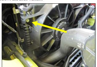
**9.** Remove the drivers side fan shroud bolt and set it aside.
