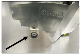
**8.** Transfer the OEM air box grommet and anti-crush sleeve into the Panel assembly as shown.
