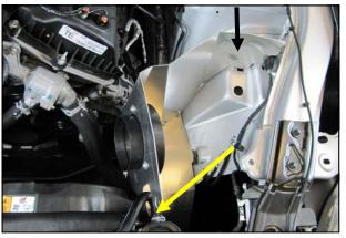
11 Install the Panel assembly into the engine compartment as shown and secure using the OEM hardware removed in steps 3 and 11.
