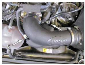
19. Connect the EVAP and crankcase vent lines to the fittings installed into the AIRAID<sup>®</sup> intake tube.
