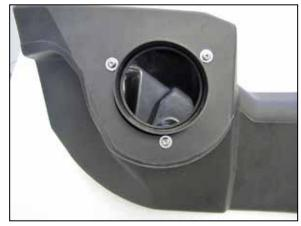
10. Install the provided filter adapter into the AIRAID<sup>®</sup> air filter housing and secure with the provided hardware.
