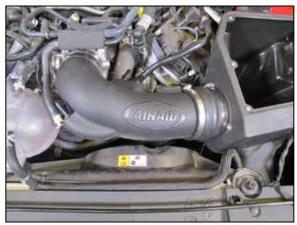
18. Install the AIRAID<sup>®</sup> intake tube into the coupler at the filter adapter and then into the coupler at the throttle body, adjust the tube for best fit and then secure with the provided hose clamps.
