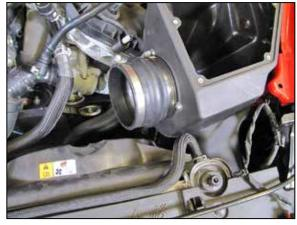
17. Install the provided hump coupler onto the filter adapter and secure with the provided hose clamp.
