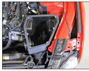
15. Install the AIRAID<sup>®</sup> air filter assembly into the vehicle and secure with the provided hardware.
