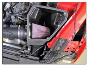
20. Install the AIRAID<sup>®</sup> air filter onto the filter adapter and secure with the provided hose clamp.
