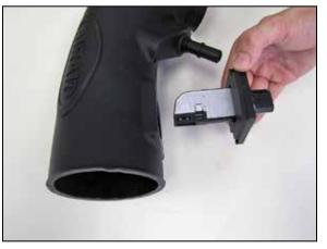
14. Install the mass air sensor assembly into the AIRAID<sup>®</sup> intake tube as shown and secure with the provided hardware.
