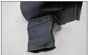
10. Remove the fresh air intake duct from the factory air filter housing and install it onto the AIRAID® air filter housing.
