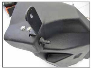
7. Install the mounting bracket and mounting stud onto the air filter housing using the provided hardware.
