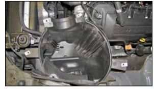
5. Remove the foam air dam, then remove the bolt that secures the factory lower air filter housing and then remove the housing from the vehicle.
