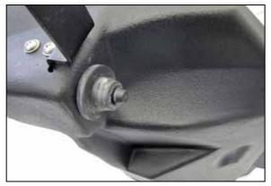
8. Install the factory air box mounting bracket onto the mounting stud installed onto the AIRAID® air filter housing in the previous step.
