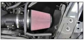
18. Install the AIRAID® air filter onto the filter adapter and secure with the provided hose clamp. Reconnect the mass air sensor electrical connection.
