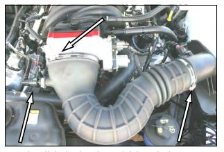
5. Reinstall the intake tube, and tighten the hose clamps.
