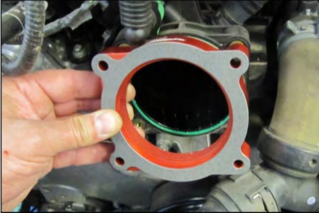
3. Install the AIRAID Spacer between the throttle body and the intake manifold with the supplied gasket next to the throttle body as shown. Make sure the “flow” arrow that is printed on the spacer is pointing towards the intake manifold.
