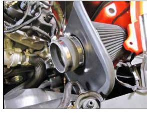
16. Install the provided hump coupler (08699) onto the filter adapter and secure with the provided hose clamp.
