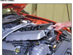
2. Lift up the decorative engine cover to dislodge it from the mounting studs and then remove the engine cover from the vehicle.
