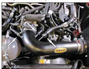
20. Connect the crank case vent, EVAP vent and idle by pass lines to the quick disconnect fittings installed into the AIRAID® intake tube.
