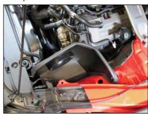
14. Set the heat shield onto the mounting bracket installed in step #10 and secure with the provided hardware.
