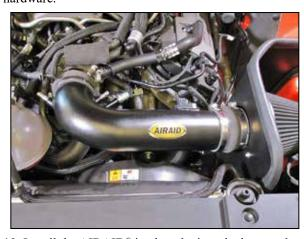
19. Install the AIRAID® intake tube into the hose at the filter adapter and then into the hose at the throttle body, adjust the tube and hoses for best fit and then secure with the provided hose clamps.
