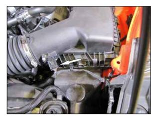
7. Release the locking tab and then disconnect the mass air sensor electrical connection.
