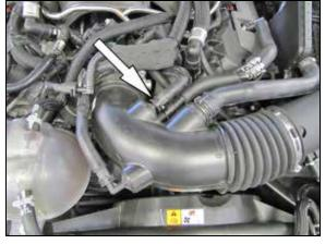
3. Depress the locking tab and then disconnect the idle bypass hose from the intake tube.
