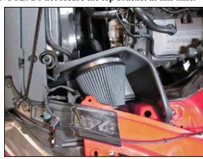
15. Install the AIRAID® air filter onto the adapter and secure with the provided hose clamp then secure the heat shield to the air filter housing mounting location using the provided hardware.
