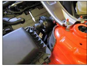
6. Install the provided cap onto the sound drum.
