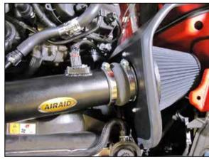
21. Connect the provided mass air sensor extension harness into the factory mass air sensor connection and then connect the other end to the mass air sensor.
