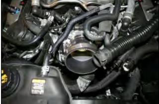
**10.** Install the Reducer and Hose clamps onto the throttle body. Place the #56 clamp on the Throttle body side of the reducer, and the #64 clamp on to the tube side.
