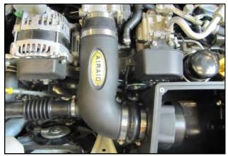
**12.** Install the Intake Tube and tighten all of the clamps. Connect the crank case breather to the Barbed Fitting and secure it using the OEM spring clamp. Insert the resonator into the Intake Tube and tighten the clamp.
