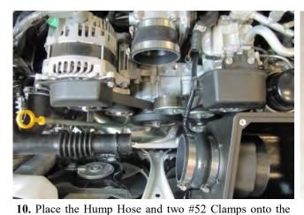
Filter Adapter and the Reducer with one #52 and one
