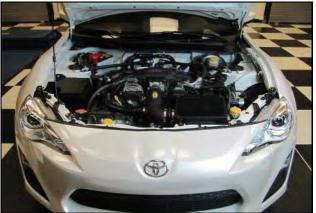
**Install Option Two: OEM air inlet removal.** While not necessary, maximum power is achieved by removing the OEM inlet from the vehicle.
