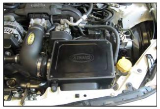
**15.** Install the Air Box Lid using the 10-24 Button Head Screws and the #10 Washers.
