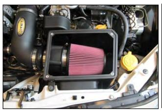
13. Install the Airaid Premium Filter onto the Filter 14 Adapter.
