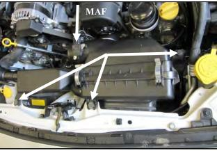
**2.** Disconnect the Mass Air Flow sensor, or MAF, in the airbox. Remove the three 6mm bolts securing the airbox assembly and remove it from the vehicle.
