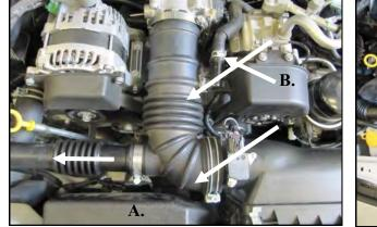
1. Disconnect The Negative Battery Terminal! Loosen the clamps on the throttle body and the airbox outlet. A. Loosen the resonator tube clamp and disconnect it from the intake. B. Compress the spring clamp on the crank case breather line and disconnect it. Remove the intake tube from the vehicle.
