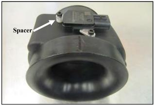
**3.** Transfer the Mass Air Flow sensor into the Filter Adapter and secure using the two 8-32 Socket Head Screws and Spacers .
