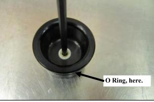
Apply a thread sealer to the threads of the Brass plug and insert it into the Resonator Tube Plug. Slide the O Ring onto the plug and into the groove. Install the Plug Assembly into the Intake tube port and secure using the #24 Clamp. It should be noted that the Aluminum Plug is designed to accept many 1/16 NPT N2O foggers.
