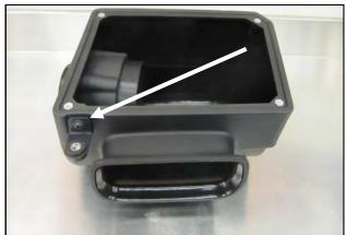
**4.** Install the Filter Adapter into the Cold Air Box as shown using the 1/4-20 Button Head Screws and 1/4" Flat Washers .
