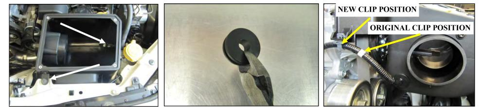
7. Slide the CAB Mount stud through the hole in the Airbox bottom and secure it using the M6 Flange Nut and a 1/4" Flat washer. Reuse one 6mm airbox bolt from step 3 to join the Airbox Bracket to the core support.
