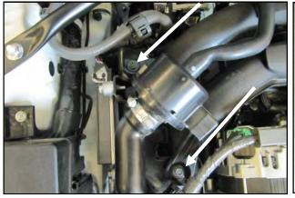
**Install Option One: Resonator Delete.** Loosen the resonator tube clamp and disconnect it from the Intake. Remove the two 6mm bolts in the diaphragm housing and pull the sound tube out of the fire wall. Remove the entire resonator as an assembly.
