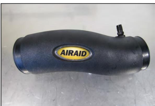
7. Install the Barbed fitting into the Airaid Intake Tube as shown. Apply the Airaid Badge to the Intake Tube as shown.
