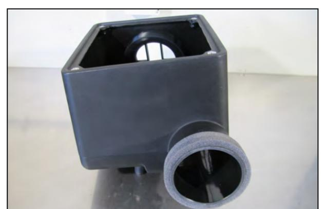
9. Prepare the Airbox inlet for Weatherstrip installation by cleaning the surface using a Prep Solvent or equivalent. Apply the self adhesive, Foam Weatherstrip onto the air inlet on the Air Box as shown. Trim any excess.
