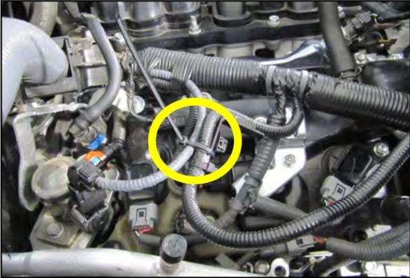
16. Use the supplied Zip Tie to tether the MAF harness to an adjacent sub harness as shown. Trim the excess length when finished.
