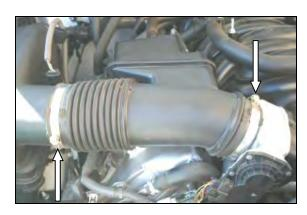
**2.** Using a 10mm socket, loosen two hose clamps on the factory intake tube. Slide the factory intake tube off of the throttle body and airbox. Move the factory intake tube aside, while leaving the factory vacuum and breather lines connected.
