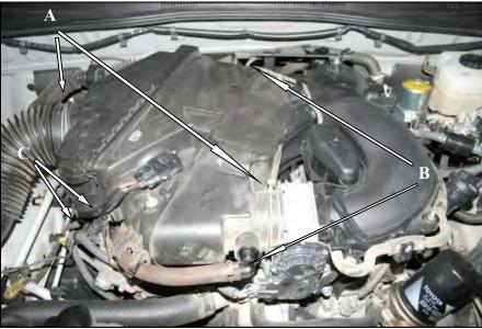
**3. A.)** Using a 10mm socket, loosen two hose clamps, one at the throttlebody, and one where the fresh air tube connects to the resonator/airbox.
