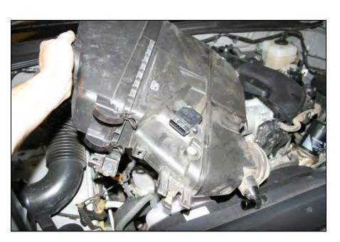
**4.** Remove the complete resonator/airbox assembly from the vehicle.
