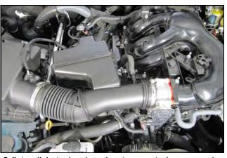
7. Reinstall the intake tube and engine cover in the reverse order in which they were removed. Re-connect the negative battery cable.
