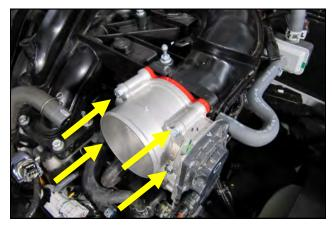
6. Reinstall the throttle body on top of the Airaid Spacer using the four bolts and washers that are supplied with the kit. Tighten the bolts evenly, in a "X" pattern.
