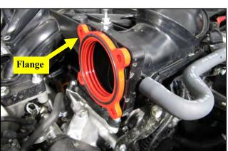
5. Insert the Airaid spacer into the intake manifold as shown. When properly installed, the O Ring flange will be facing outward.
