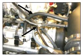
**10. 03-04 Tundra Pickup & 04 Sequoia** A) Install the 1/2"x 13" breather hose (#5) from the MIT to the valve cover. B) Install the 1/4"x1/4"x1/8" vacuum tee (#9) into the 1/4"x4" hose (#8) and then to the factory 1/4" and 1/8" vacuum lines, as shown.
