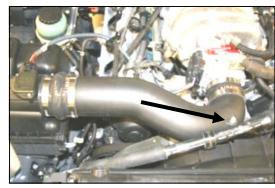
**9.** Install the MIT into the hump hose first, and then into the reducing coupler. Adjust the MIT snugly against the throttle body, and tighten the 4 hose clamps. Next install the supplied button head bolt (#12) and washer (#11) thru the Adel clamp and into the MIT to hold the air conditioning hose.
