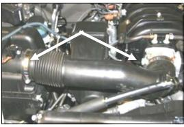
**3.** Loosen the hose clamps on the intake tube at the throttle body, and at the airbox.
