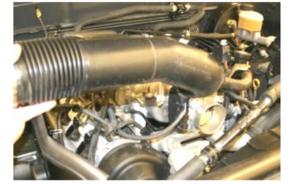
**4.** Remove the factory intake tube from the vehicle.
