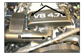
1. **Disconnect negative battery cable.**A) Remove two 10mm nuts, and remove beauty cover. (Save for reuse). B) Remove the bolt thru the Adel clamp that holds the air conditioning
