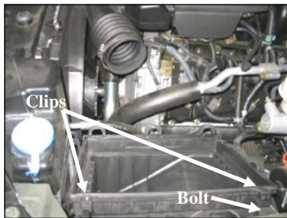
2. Unclip the factory air box lid from the factory air box base, and remove it from the engine compartment. Remove the factory air filter from the air box base. Using a 10mm socket, remove two bolts (three on some vehicles) from the air box base (save for reuse).
