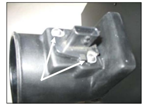
6. Using two 8-32 x 1/2" SS button head screws (#11), reinstall the factory MAF sensor into the air filter adapter.
