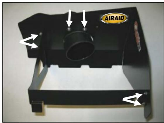
5. Assemble the Airaid Quick Fit Panels (#2, #3) using four 6-32 x 5/16" screws (#6), #6 flat washers (#7), and 6-32 keps nuts (#8). Next, install the air filter adapter (#4) using two 1/4-20 x 1/2" button head bolts (#9), and 1/4" flat washers (#10).
