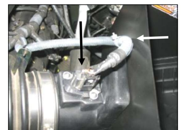
9. Reconnect the MAF sensor wiring harness to the sensor. Mount the factory wiring harness clip into the hole in the Airaid Quick Fit panel.
