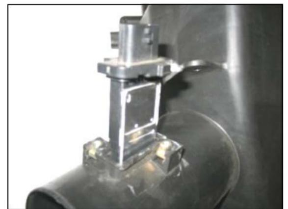
3. Using a Phillips head screwdriver, remove two screws and the MAF sensor from the factory air box lid. Save the sensor for reuse.
