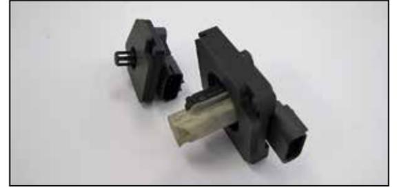
16. Install the factory sensors into the provided sensor adapters and then install the provided gaskets onto the adapters.
