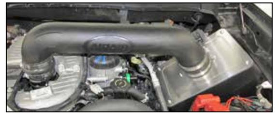
18. Install the AIRAID® intake tube assembly into the coupler at the turbo and filter adapter, adjust the tube for best fit and then secure with the provided hose clamps.
