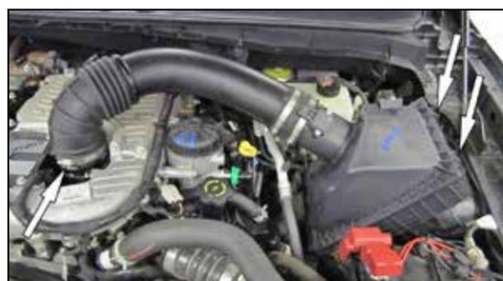
3. Loosen the hose clamp that secures the factory intake tube to the turbo inlet. Release the clips that secure the upper air filter housing to the lower housing and then remove the upper housing and intake tube from the vehicle.
