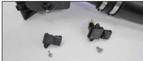
15. Remove the mass air sensor and temperature sensor from the factory air filter housing.
