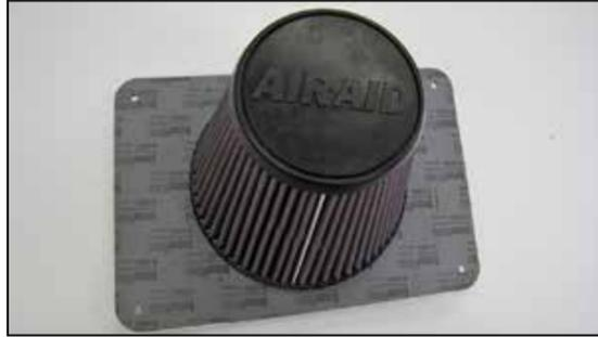
11. Place the housing lid gasket onto the lid and then install the AIRAID® air filter and secure with the provided hose clamp.
