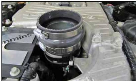
14. Install the provided hump coupler onto the turbo inlet and secure with the provided hose clamp.
