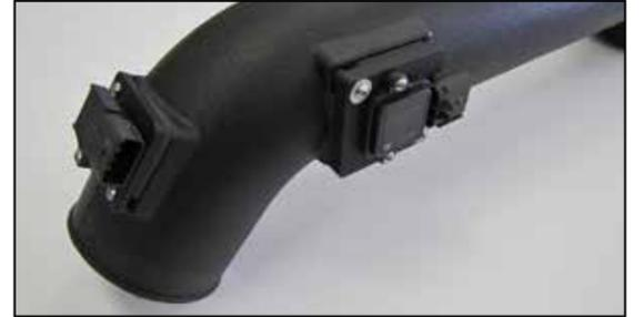
17. Install the sensor assemblies into the AIRAID® intake tube and secure with the provided hardware. **NOTE: Be sure the mass air sensor is installed in the correct direction.**
