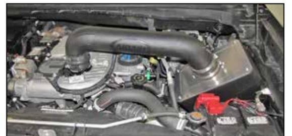
**20. Double check your work!** Make sure there is no foreign material in the intake path. Make sure all clamps, hoses, bolts, and screws are tight. Double check the hood clearance! **Reconnect the negative battery cable!**
