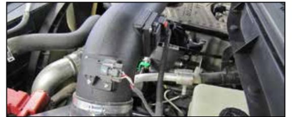
19. Reconnect the mass air and temperature sensor electrical connections.
