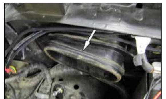
5. Remove the gasket from the factory fresh air intake.
