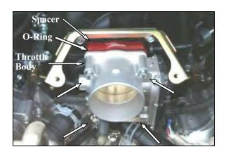
3. Install the O-Ring (#2) into the groove on the Airaid Spacer (#1). Install the spacer between the intake manifold, and the throttle body with the O-Ring facing the throttle body. Insert four 6mm x 70mm Hex Bolts (#3), and 6mm Flat Washers (#4) through the throttle body, Airaid Spacer, and into the intake manifold. Using a 10mm socket, tighten all 4 throttle body bolts evenly, to the manufacturer's specifications.
