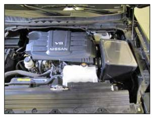
22. Double check your work! Make sure there is no foreign material in the intake path. Make sure all clamps, hoses, bolts, and screws are tight. Double check the hood clearance! Reconnect the negative battery cable!
