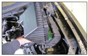
4. Unclip and remove the air filter housing lid.
