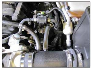
18. Install the hose menders into each vent hose and then connect the hoses to the factory vent hoses and to the fittings installed into the AIRAID<sup>®</sup> intake tube.
