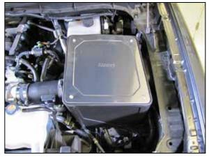
19. Install the air filter housing gasket and lid and secure with the provided hardware.
