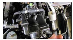
6. Disconnect the crank case vent lines and then loosen the clamp that secures the canister to the intake tube and remove the canister.
