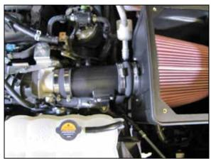
16. Install the provided hump coupler onto the AIRAID<sup>®</sup> intake tube and then install the intake tube into the vehicle, adjust the tube for best fit and then secure with the provided hose clamps.
