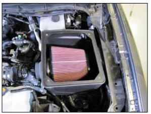
15. Install the AIRAID<sup>®</sup> air filter housing into the vehicle and then install the air filter onto the filter adapter and secure with the provided hose clamp.
