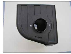
9. Install the filter adapter into the AIRAID<sup>®</sup> air filter housing using the provided hardware.
