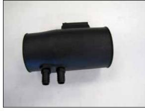
13. Install the two vent fittings into the AIRAID<sup>®</sup> intake tube as shown.
