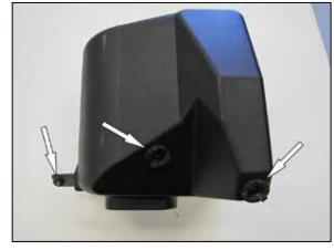
10. Remove the three mounting grommets from the factory air filter housing and install them into the AIRAID<sup>®</sup> housing as shown.
