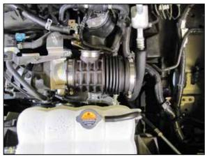
7. Loosen the hose clamp and then remove the factory intake tube from the vehicle.
