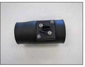
12. Install the mass air sensor assembly into the AIRAID<sup>®</sup> intake tube and secure with the provided hardware.
