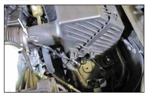
2. Disconnect the mass air sensor electrical connection and then unclip the harness from the air filter housing.
