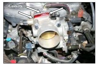
4. Install the spacer (#1) (*with the flat side of the helix bore facing the throttle body*) between the intake manifold, and the throttle body with one of the supplied gaskets (#2) on each side of the spacer. Insert four 8mm x 75mm Hex Bolts (#3), and 8mm Flat Washers (#4) through the throttle body, Airaid Spacer, and into the intake manifold. Using a 13mm socket, tighten all 4 throttle body bolts evenly, to the manufacturer's specifications.
