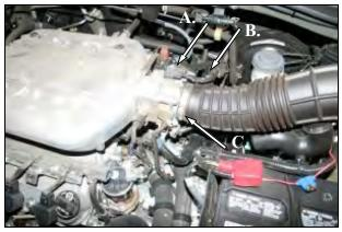
2. A.) Disconnect the wiring connector on the top of the throttlebody. B.) Squeeze the clamp with your fingers and disconnect the metal tube from the intake tube. C.) Using a 10mm socket, loosen the hose clamp on the throttle body end of the factory intake tube. Pull the intake tube out from between the throttle body and the airbox and set it out of the way.
