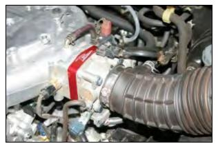
5. Reinstall the factory intake tube, and tighten the hose clamp. Reconnect the metal tube to the intake tube. Reconnect the throttle body wiring connector. Reinstall the engine beauty cover. **Re-connect the negative battery cable!**
