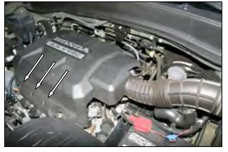
1. **Disconnect the negative battery cable!** Using a flat blade screwdriver, turn the plastic keepers at the front of the engine beauty cover. Remove the engine beauty cover by lifting up and releasing it from the grommets.
