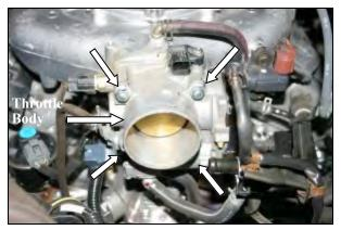
3. Remove the two nuts and two bolts that secure the throttle body to the intake manifold. Remove the throttle body and the factory gasket. Remove the two studs that are left in the intake manifold.
