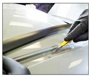
17. Using a knife, slice the sealing tape to allow access to the inserted nuts. NOTE: Do not remove the tape, slicing the tape will allow the bolt to pass through.
