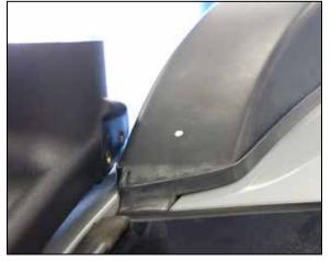
23. On vehicles equipped with a factory TOYOTA roof rack, intall the snorkel onto the fender with the provided top bracket. Mark the location for the hole to be drilled into the roof rack.
