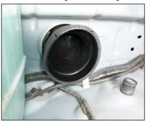
31D. Install the flexible spacer into the flexible duct as shown and then the AIRAID air filter housing can be installed.
