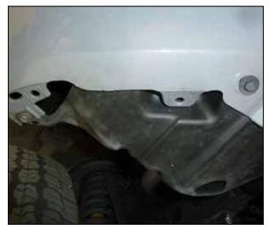
29. Replace the two inner fender retaining clips with the clips provided and then reinstall the two factory screws.
