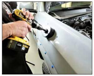
14.Drill three <sup>1</sup>/<sub>2</sub>" holes for the snorkel mounting location and using a 4" hole saw, drill the 4" hole for the air duct. NOTE: the 4" hole will be drilled through different angled surfaces, use caution while drilling to not distort the remaining sheet metal.
