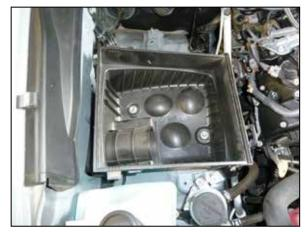
31. Reinstall the lower air filter housing and secure with the factory hardware. Secure the snorkel duct to the air filter housing with the provided hose clamp. **NOTE: It may be necessary to move the washer bottle to gain access and tighten the hose clamp.**
