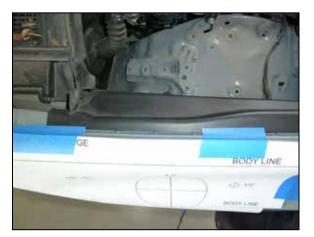
12. Cut the hole template provided and tape together. Tape the assembled template to the front fender as shown. Using the template guide, mark the four locations in the fender that will be drilled with a center punch or similar device. NOTE: The fender sheet metal is thin, light tapping is all that is needed to mark the hole location.
