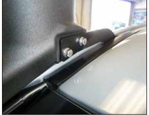
22. **On vehicles without a factory TOYOTA roof rack**, install the snorkel onto the fender and secure it to the top mounting bracket with the hardware provided.
