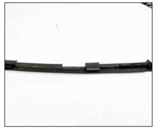
19. Set the roof trim back in position and note where the bracket interferes with the trim. Using side cutters or a razor blade, trim the roof trim so that it will lay flat back into the channel and around the bracket.
