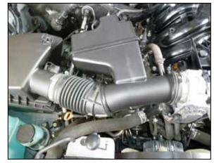
33. Reinstall the intake tube and secure with the factory hose clamps. Reconnect the vent lines.
