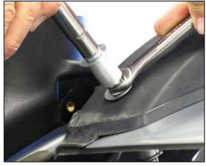
26. Using a 9/16" wrench to hold the nut and a 10mm socket and ratchet to tighten the bolt while applying downward pressure on the bolt. This compress the Rivnut and grip the plastic of the roof rack. Tightening force will be high initially and then lessen until the Rivnut is set. Force will ramp up again once set, do not over tighten.
