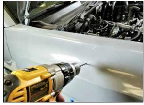
13. Drill a 1/8" pilot hole in all four locations to be drilled.
