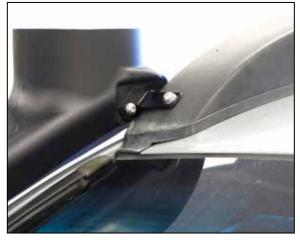
27. Install the upper mounting bracket and secure with the provided hardware.
