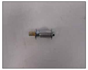
25. If a Rivnut setting toll is not available, assemble the provded hardware as shown to istall the Rivnut. **NOTE: The nut passes over the threads of the bolt, it does not thread on.**
