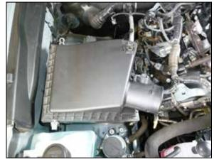
32. Install the air filter and upper housing.
