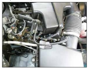
34. Reconnect the mass air sensor electrical connections and secure the wiring harness.
