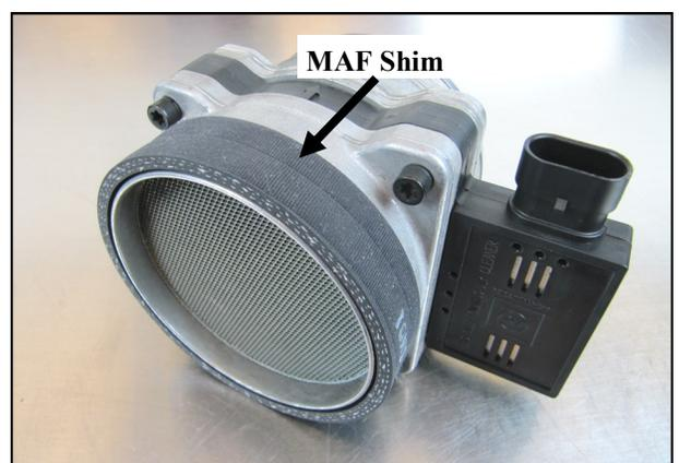
4. On 1997-2000 models the MAF shim will need to be installed for proper fit.
