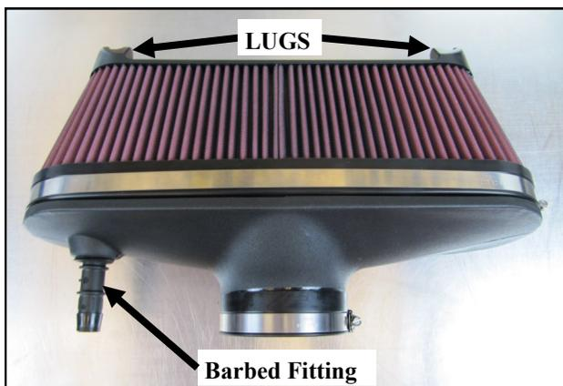
3. Create the Filter Assembly as shown using the supplied Grommet, Barbed Fitting and Hose Clamps. Refer to the Exploded Diagram for assembly detail. Note the location of the Filter location lugs and their position relative to the Barbed Fitting. Maximum Hose Clamp torque is to be no greater than 20 LB/IN.
