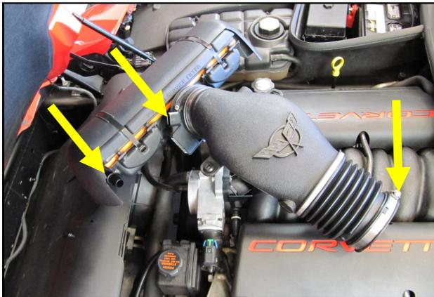
1. Disconnect the Mass Air Flow sensor, the air pump breather line and loosen the hose clamp on the throttle body. Remove the entire intake as an assembly and set it aside.
