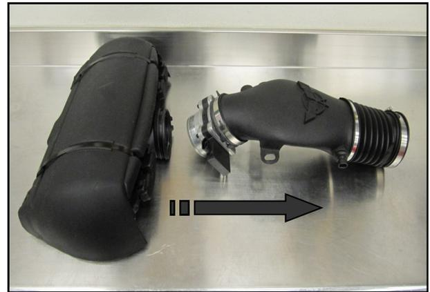
2. Separate the factory air box from the intake tube and Air Flow meter.
