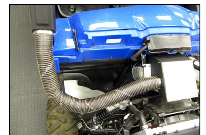
36. Full view of Duct routing. Duct is provided with additional 8" in length and may be trimmed if desired.
