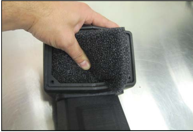
25. Carefully insert the Airaid Foam Prefilter (#6) into the Snorkel Inlet.
