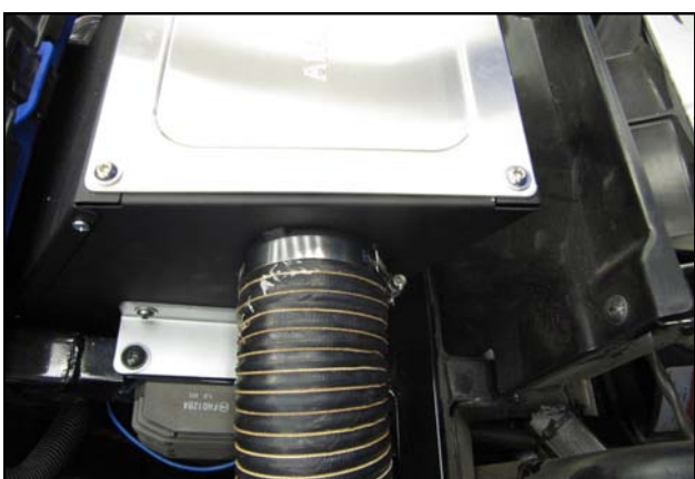
34. Install the Flexible Duct onto the Airaid performance airbox as shown using a #48 Clamp.
