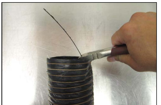
33. Using a pair of dykes, pull out approximately three windings of the steel wire inside of the Ducting (#16) and cut it off.
