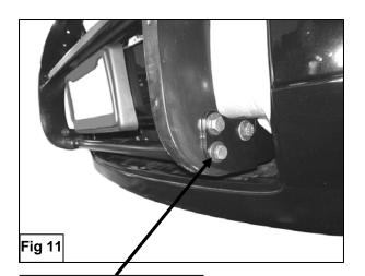
12mm x 35mm Hex Bolts 12mm Lock Washers 12mm Hex Nuts 12mm Flat Washers
