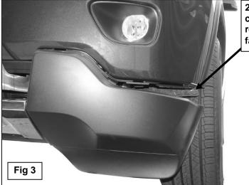
2011-13 vehicles: Remove factory hardware and release clips at ends of lower bumper cover only. Do not remove lower bumper cover. (For vehicles without factory tow hooks only)
