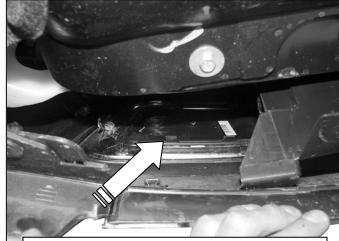
(Fig 8) 2014 driver side pictured from below front bumper. Carefully pull the air dam slightly forward and reach up between bumper cover and radiator support to access and remove block offs
