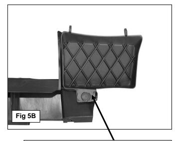
Remove (2) factory clips to remove the block off cover from each end of the air deflector. 2011-13 driver side of air deflector pictured
