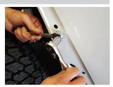
Place the fender back into place, and attach using an M6 bolt, lock washer and flat washer.
