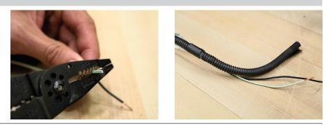
Remove approximately 4" of the flex wire cover from the prepared end of the wiring harness.
